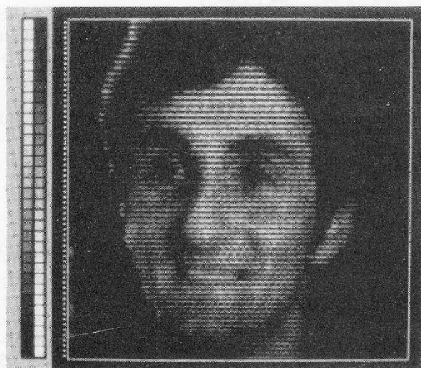
Fig. 6. Scene of Fig. 4, but using a doubled, 2.10 s, conversion time with the linear frequency distribution.
