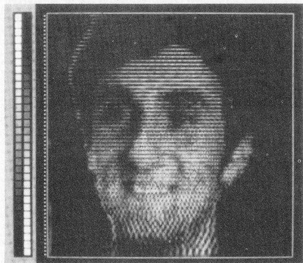
Fig. 10. Scene of Fig. 4, but using an exponential frequency distribution and a doubled, 2.10 s, conversion time. The vertical axis is logarithmically compressed.
